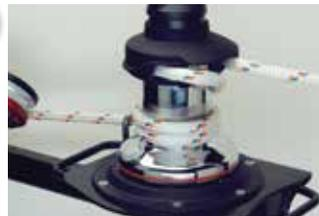
**Warning:** Take at least two turns of the rope around the winch drum. If it slips under load, increase the number of turns to a maximum of four, taking care not to overlap the rope.
