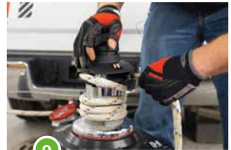
9 Insert the rope into the rope grab. Raise the cover for ease.
