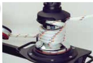
**NOTE!** The number of turns needed around the winch drum depends on the load and the condition of the rope. Check the device's descending capacity in its working configuration.
